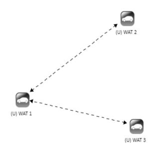
In the step above, we purposefully made an error. We should have drawn a uni-directional. not a bi-directional link from WAT3 to WAT1. Now we want to delete that link.
